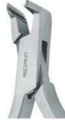
LD33-106 Distal End Cutter Universal cut Box Joint 12cm Max: .021"(.54mm) x .025"(.64mm) Min: .012"(.31mm)
